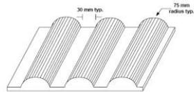
Figure 1. Crush test textured planar surface.
