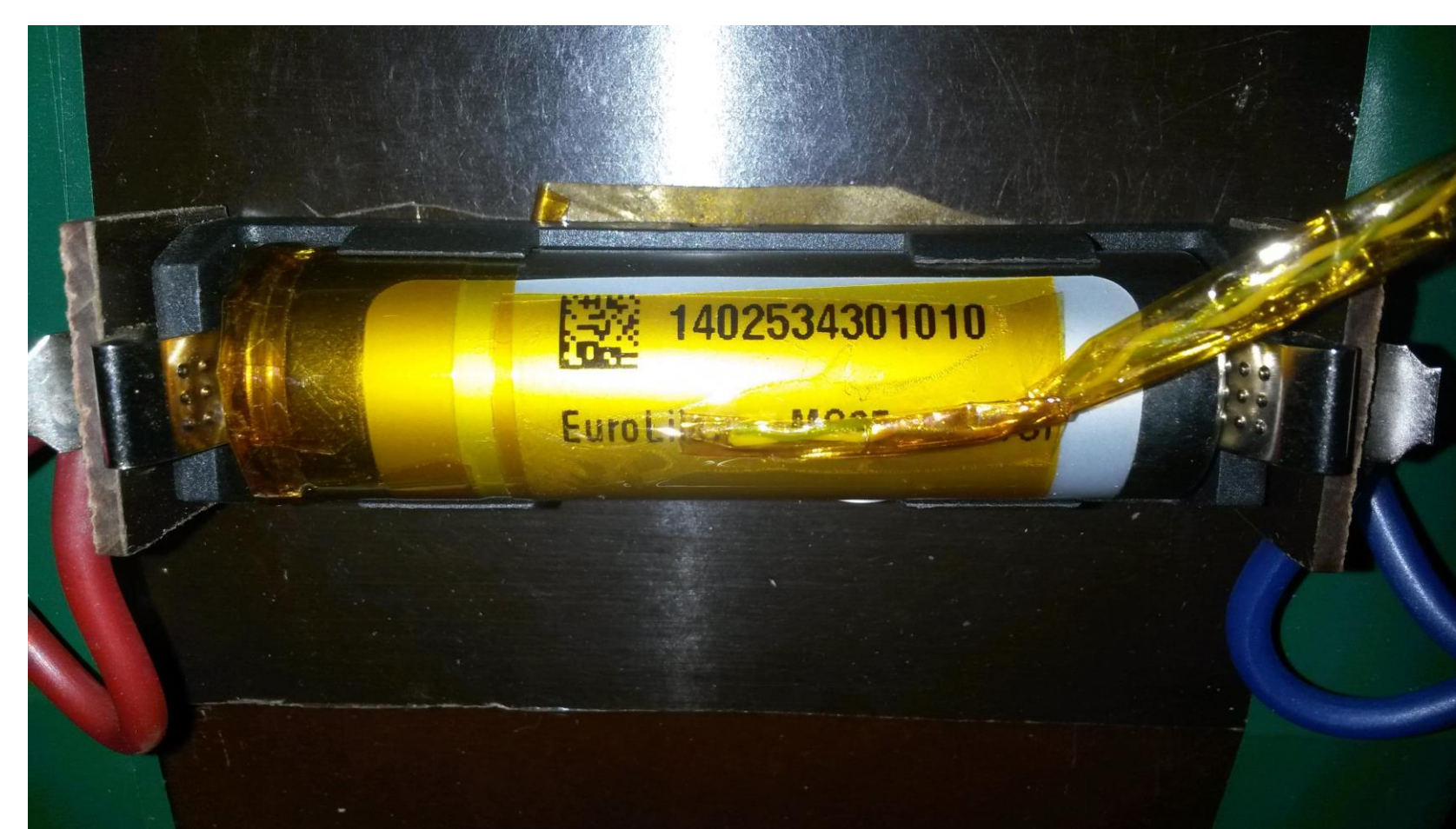
EuroLiion LFP/Si 18650 cell Gen. I in test frame
