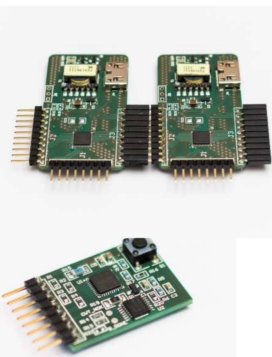
Test boards for with AS8506; Stackable or standalone board for autonomous battery balancing
