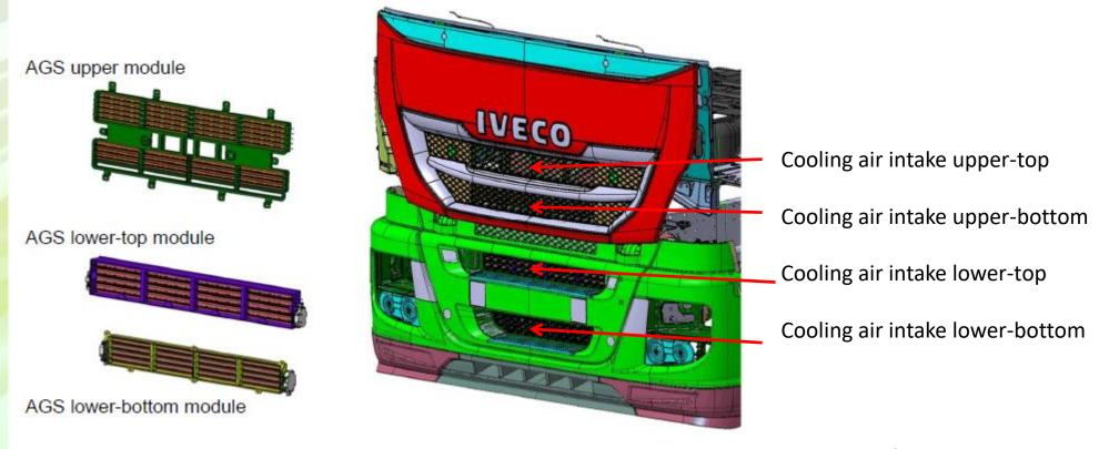
A feasibility study of Active Grille Shutters has been performed, including packaging/installation study .The AGS system has resulted to be a quite promising solution for reducing the aerodynamic drag coefficient in the front part of the vehicle.
