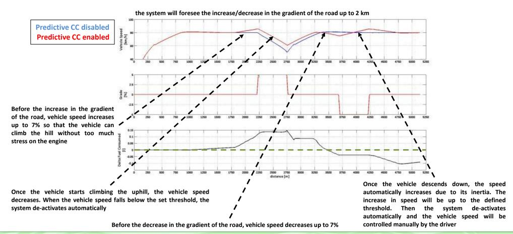
Use case: Hybrid Vehicle with e-Powertrain (139 kW 1050 Nm EM + 26 kWh HV battery)
