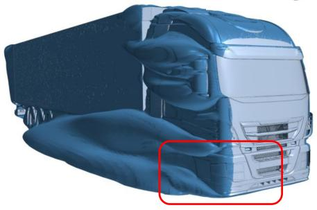
The blue image illustrates how the more rounded corner and the channel, together with the extended door, induce the flow to move closer to the surface.
