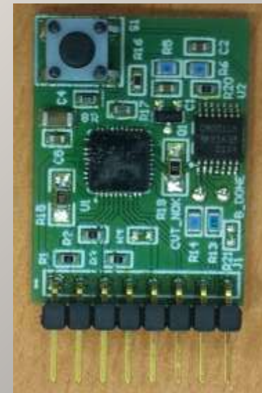
Test board for autonomous battery balancing with AS8506
