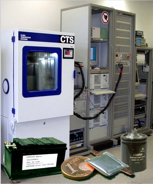
Testbench ( \pm 600A ; -5V to +60V ) with climate chamber ( -70^{\circ}C to +180^{\circ}C )
